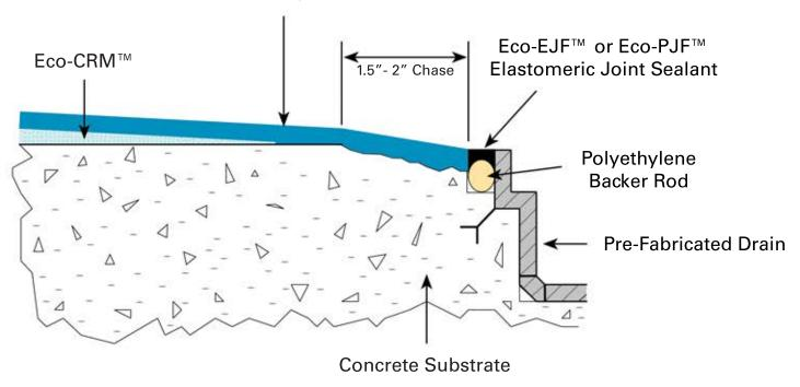
**Note**: Backing Rod positioned to provide an installed sealant depth that is equal to 50% of the joint width.
