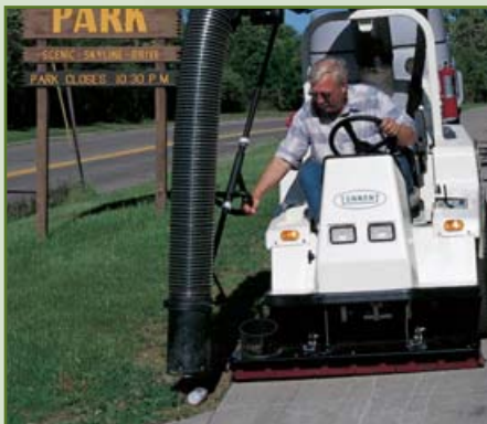
The ATLV removes litter, cans, and broken glass from grass-covered grounds in parks or stadiums.
