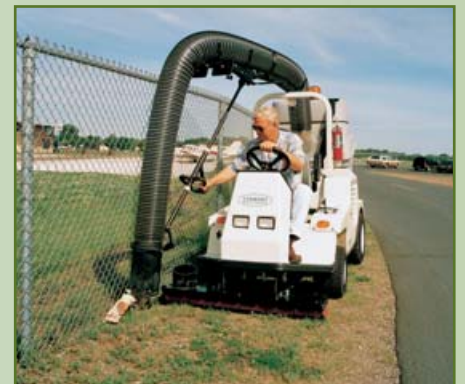
Vacuum nozzle with adjustable handle reaches to clean thoroughly alongside fences.
