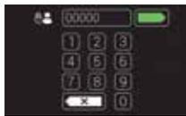
**Pro-ID™** gives the supervisor the ability to program the machine to the skill level of the operator and helps prevent unauthorized use.
