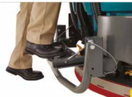
Recovery Tank Access Step
