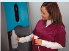
Through the process of electrolysis, the Orbio 5000-Sc creates a multi-purpose cleaning solution on site using tap water, salt, and electricity. The 5000-Sc solution effectively replaces many conventional daily-use cleaning chemicals.
