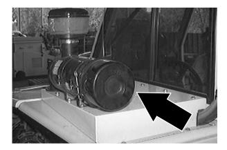
Install the dust cap on the air filter housing with the arrows pointing up. (For machines below serial number 006009)
