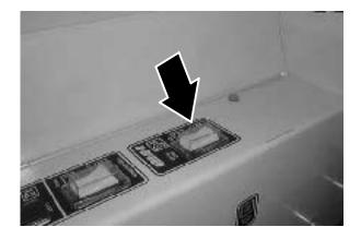
3. Press the filter shaker switch to shake the hopper dust filter.
