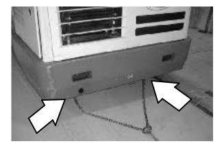
The rear tie-down locations are through the U-bolt section of the main frame under the side bumpers toward the rear.
