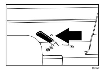
Idle: Push the lever into the **Idle** position. This speed is for idling.
