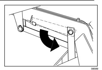
5. Slowly lower the hopper so the support bar rests on the bar stop on the machine frame.
