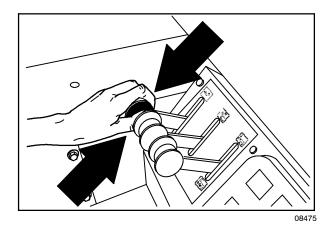
Close: Push and hold the hopper door lever in the **Close** position.
