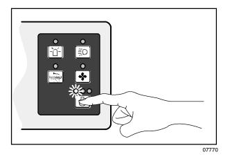
Idle: Press the engine speed switch until the second indicator light comes on. This speed is for idling.
