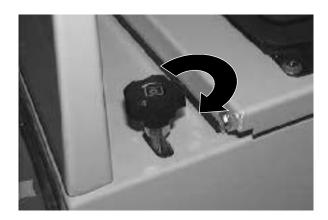
If the main brush pattern is tapered, more than 15 mm (0.5 in) on one end than the other, adjust the taper at the drive end of the brush.
