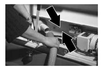
9. Close the vacuum door by sliding the vacuum door lever down and to the left into the locked position.
