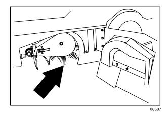
*Crinkle Wire 8-double Row Main Brush* – The stiff wire bristles cut through compacted grime, hard to sweep dirt, and dirt mixed with oil, grease, or mud. This brush is recommended for foundry sweeping where heat may melt synthetic bristles. This brush has good hopper loading ability, but is not recommended for dusty applications.
