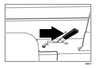
3. Turn the key counter-clockwise. The glow plugs light will come on. Hold the key in this position for 15 to 30 seconds, depending on weather conditions. Colder weather requires longer time.
