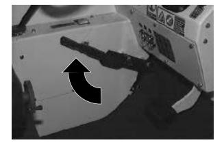
2. Turn off the vacuum fan by pressing the vacuum fan switch. The indicator light above the switch will go off.
