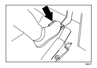
3. Select the **Idle** position with the engine speed switch. (For machines below serial number 006009)
