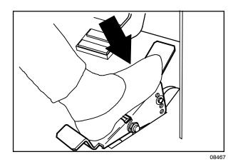
Reverse: Press the bottom of the directional pedal with the heel of your foot.
