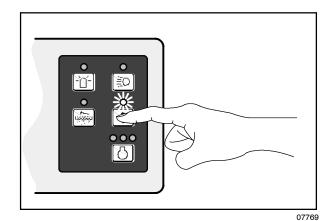
3. Turn off and lift the main brush by placing the switch in the middle **Off** position.
