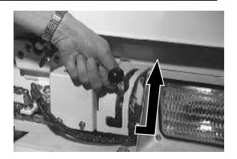
14. Disconnect the vacuum hose from the vacuum adaptor tube in front of the hopper.
