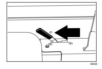
3. The hopper door has to be closed during sweeping. If your machine has the hopper door light option, make sure the hopper door light is off. If the hopper door light is on, close the hopper door.
