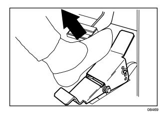
The toe angle of the directional pedal is adjustable. Remove the clevis pin, move the top of the pedal to the angle needed, and put the clevis pin through the adjustment holes.
