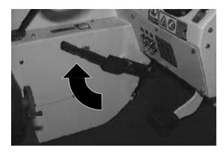
Turn the ignition switch key counter-clockwise to stop the engine. Remove the switch key.
