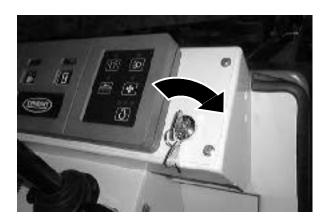
4. Turn the ignition switch key clockwise until the engine starts.
