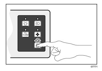
Fast: Press the engine speed switch until the third indicator light comes on. This speed is for sweeping.
