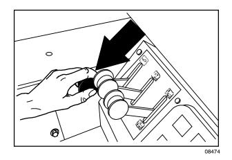
Hold: Release the hopper door lever into the middle position.
