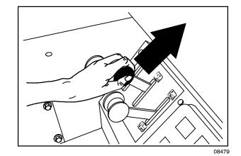
12. Push and hold the hopper lift lever in the **Down** position.
