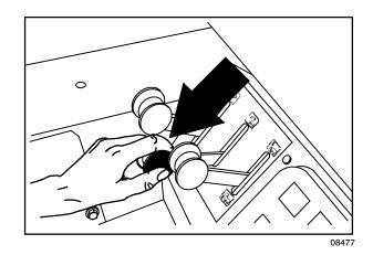
Hold: Release the hopper rollout lever into the middle position.
