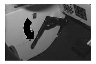
7. Select the **Fast** engine speed with the engine speed switch. (For machines below serial number 006009)
