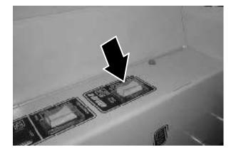
4. Turn off and lift the side brush(es) by placing the bottom of the switch(es) into the **Off/Up** position.
