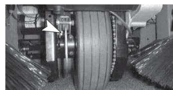
5. Check condition and tension of belts and chains. Lubricate the chains with SAE 30 Engine oil.
