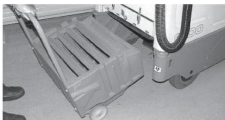
4. Make sure the hopper dust filter is properly installed and clean.
