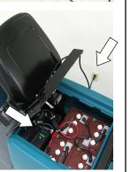
**Connect the battery to the charger** and plug in every day after use or
