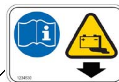
FOR SAFETY LABEL - Read manual. Battery compartment drain hose. Avoid contact with battery acid. Located above battery compartment drain hose.
