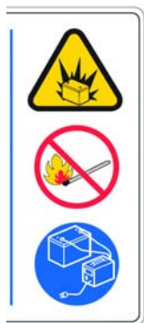
WARNING LABEL - Batteries emit hydrogen gas. Explosion or fire can result. Keep sparks and open flame away when charging.
