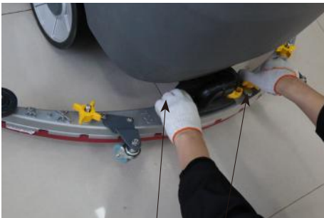
Unscrew the fixing nut counterclockwise
