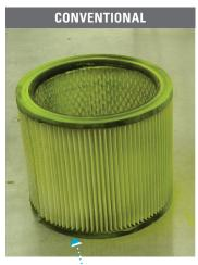
Dust embedded in the filter is harder to clean off and shortens the filter life
