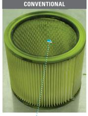
Yellow particles can be seen inside the filter, clogging the filter membrane
