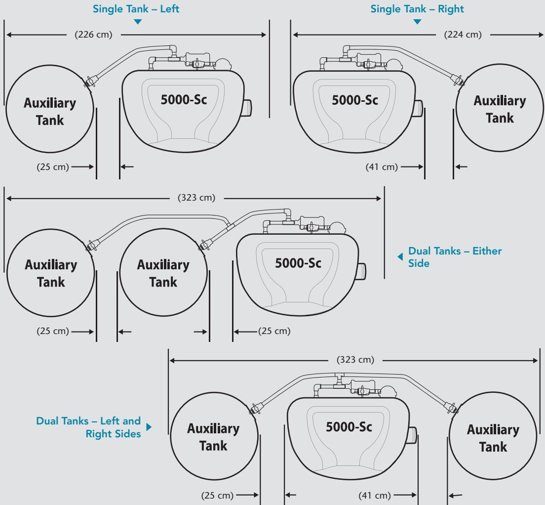
5000-Sc unit and any auxiliary tanks should be installed on an even surface so that the bases of a complete installation are at the same level. A 40,64 cm gap is required between an auxiliary tank and the right (inflow filter) side of the tank to allow for access to the inflow filter.
