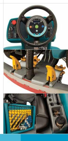
Effectively clean along edges with the scrubbing side brush that expands cleaning path for maintenance cleaning productivity. Bring high performance spill recovery to hard-toreach areas with the in-line telescoping vac wand. Reduce repair costs and protect the rear squeegee when backing up with the rear squeegee protection kit Protect operators from falling objects with the overhead guard and protect the T16 from contact damage with the severe environment front bumper.
