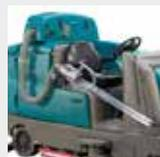
**Live wand** quickly picks up miscellaneous lightweight debris like shrink wrap.
