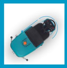
Compact and Maneuverable Design Reach many areas of the facility and narrow spaces with the highly maneuverable scrubber with a 1m turning radius and front-mounted drive design.
