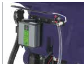
Solution tank level gauge and drain hose
