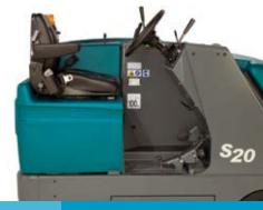
Improve productivity with a 62 in / 1,575 mm sweeping path that shortens cleaning time by adding optional dual side brushes and a high-capacity debris hopper.
