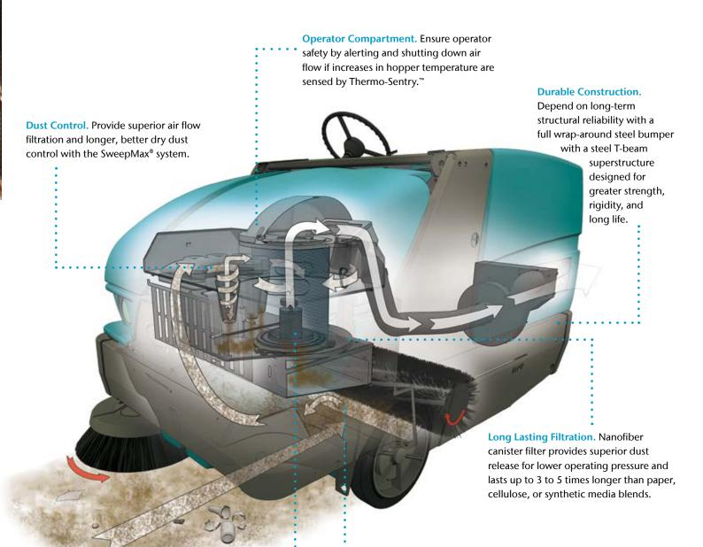
**Simple Filter Cleaning.** Increase ••••• efficiency with the ShakeMax® 360 °filter cleaning mechanism, dislodging dust particles caught deep within the pleats.
