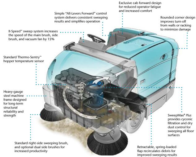
Reduce downtime and operator fatigue with easy no-tool brush removal and change, aided by the self-guiding 8-spline drive and idler hub
