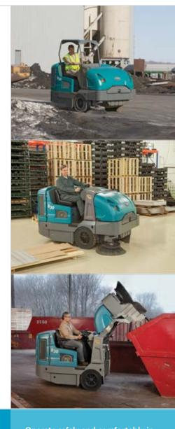
Achieve outstanding results in diverse environments with dual side brushes which, combined with a large 14 ft<sup>3</sup> / 395 L Duramer™ hopper, allow you to sweep up to 80 in / 2,030 mm in a single pass.
