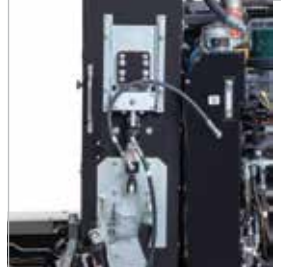
传送带张力自我调节设计 CONVEYOR SELF-TENSIONING
